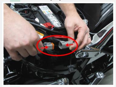
Connect Diag4bike to motorcycle and make sure, that the battery is well charged. For sure you can connect battery charger.
