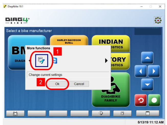
Fig. 37 – Analog measuring configuration is started by clicking the configuration icon (pos 1) and confirming it (pos 2) (illustrative picture)
