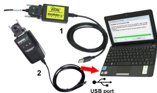
Fig. 16 – Information window with a request to connect VCI communication interface to computer (1 - AT531 5074, 2 - AT532 5006)
