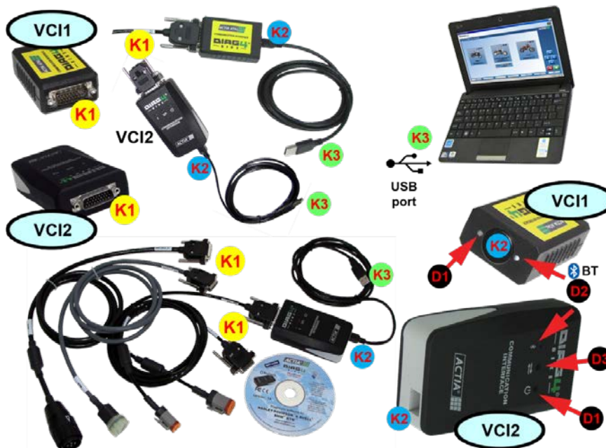
Fig. 20 – Description and connection of the VCI communication interface
