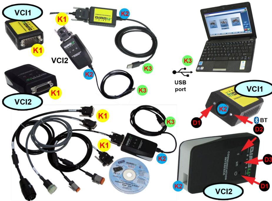
Fig. 20 – Description and connection of the VCI communication interface (1 - AT531 5075, 2 - AT532 5007)
