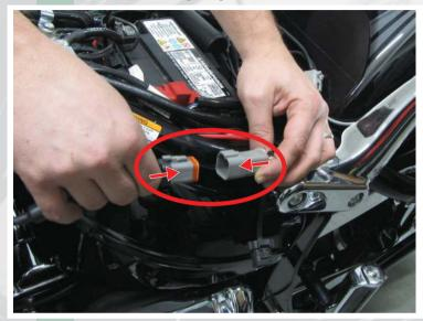
Connect Diag4bike to motorcycle and make sure, that the battery is well charged. For sure you can connect battery charger.
